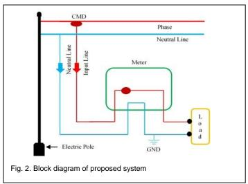
The current measuring devices are connected at the supply
