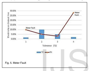
value. When the  $f_m$  value is more than the tolerance value of output line of meter (T<sub>2</sub>) then occurs the meter fault. Set-1 and set-4 show in Fig. 5 indicated the meter fault.
